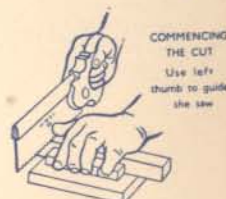
CROSS CUTTING Support the outer end with left hand
